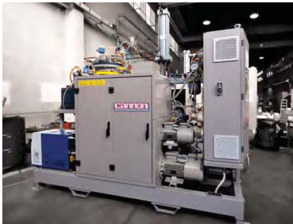
Each Component has a Dedicated Thermoregulator
